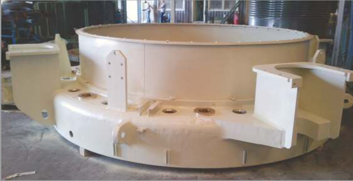
Montajlı Ayar Ringleri (24 Ton) / Assembled Adjustment Rings (24 Tons)
