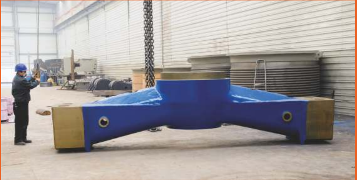
Primer Kırıcı Üst Kolu (28 Ton) / Gyratory Crusher Spider (28 Tons)
