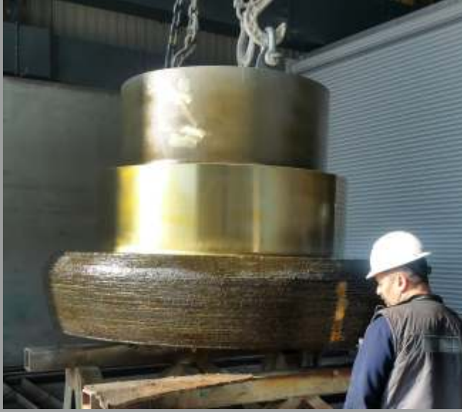
Sert Dolgulu Roller / Roller With Hardfacing
