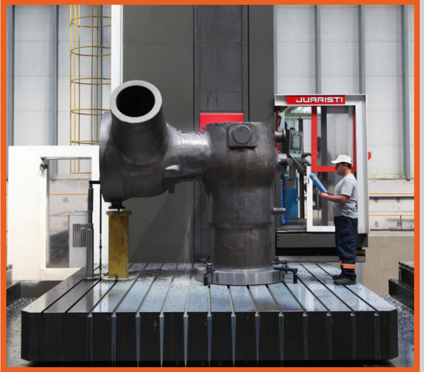
Valve Casing / G17CrMoV5-10
