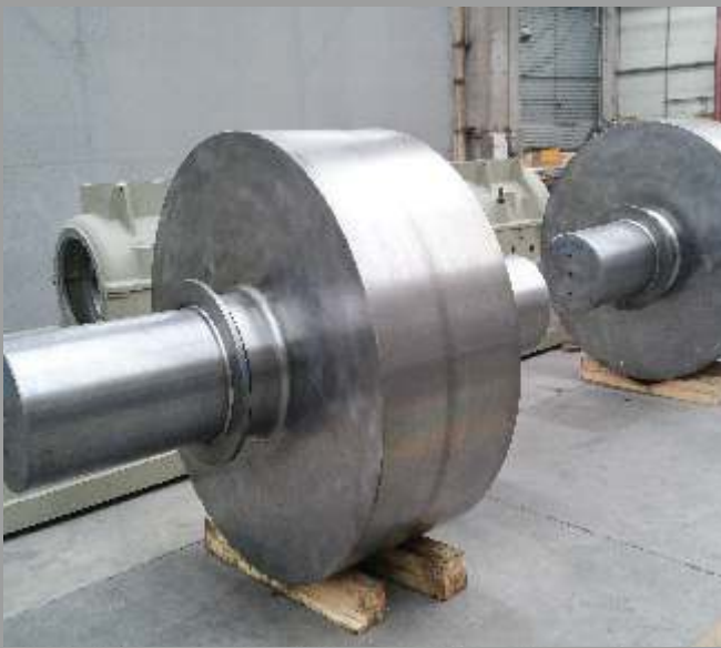
Montajlı Gale (57 Ton) / Assembled Roller (57 Tons)
