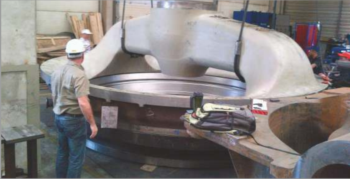
Primer Kırıcı Kolu (47 Ton) / Gyratory Crusher Spider (47 Tons)
