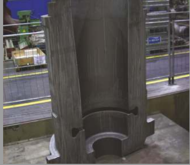
Guide Blade Carrier / G17CrMoV5-10
