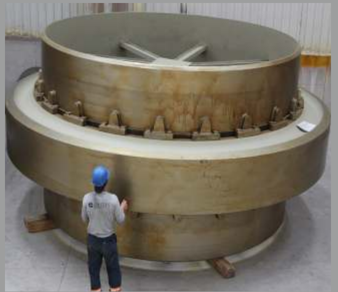
Fırın Ringi (56 Ton) / Kiln Tyre (56 Tons)
